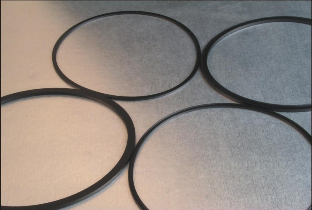
Rubber back-up ring (80 Shore A) is usually used with O-ring in order to bear greater pressure. Customer can order according to the size of o-ring for convenience.
